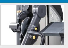
Dual cam system improves biomechanics and reduces cable slack
